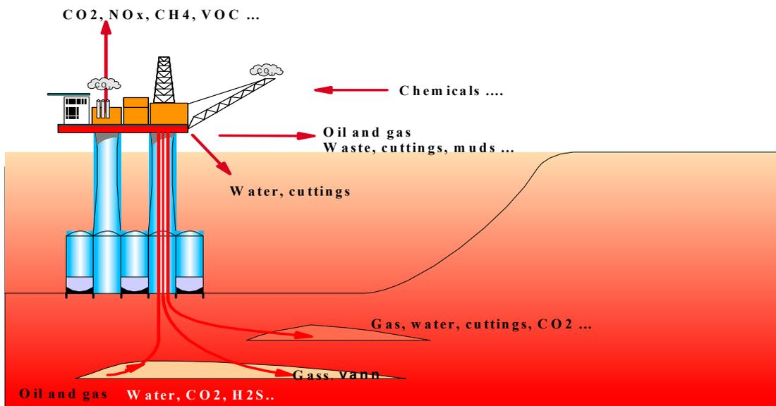
Figure 3. Emissions from an oil platform (Adopted from Johnsen [www.naturvern.no/data/f/0/69/90/3\\_2401\\_0/Statoil](http://www.naturvern.no/data/f/0/69/90/3_2401_0/Statoil)).
